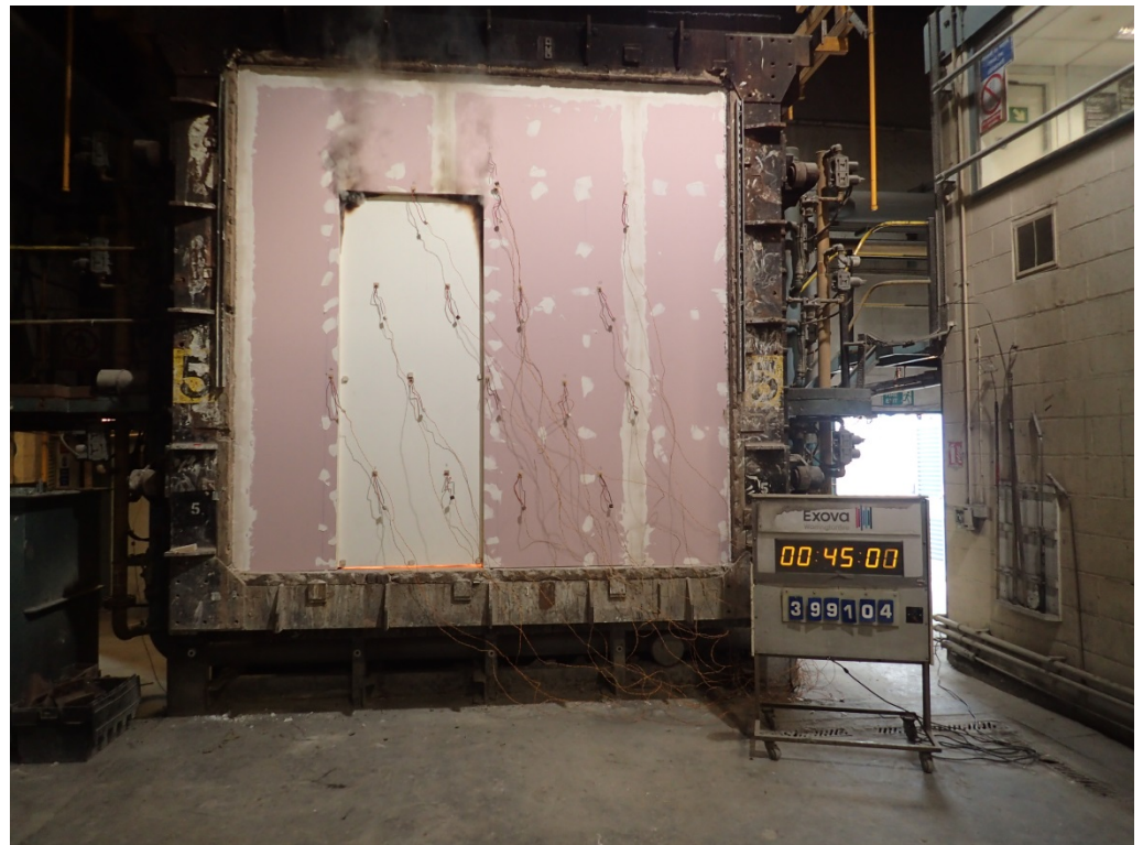
The unexposed face of the test construction after a test duration of 45 minutes
