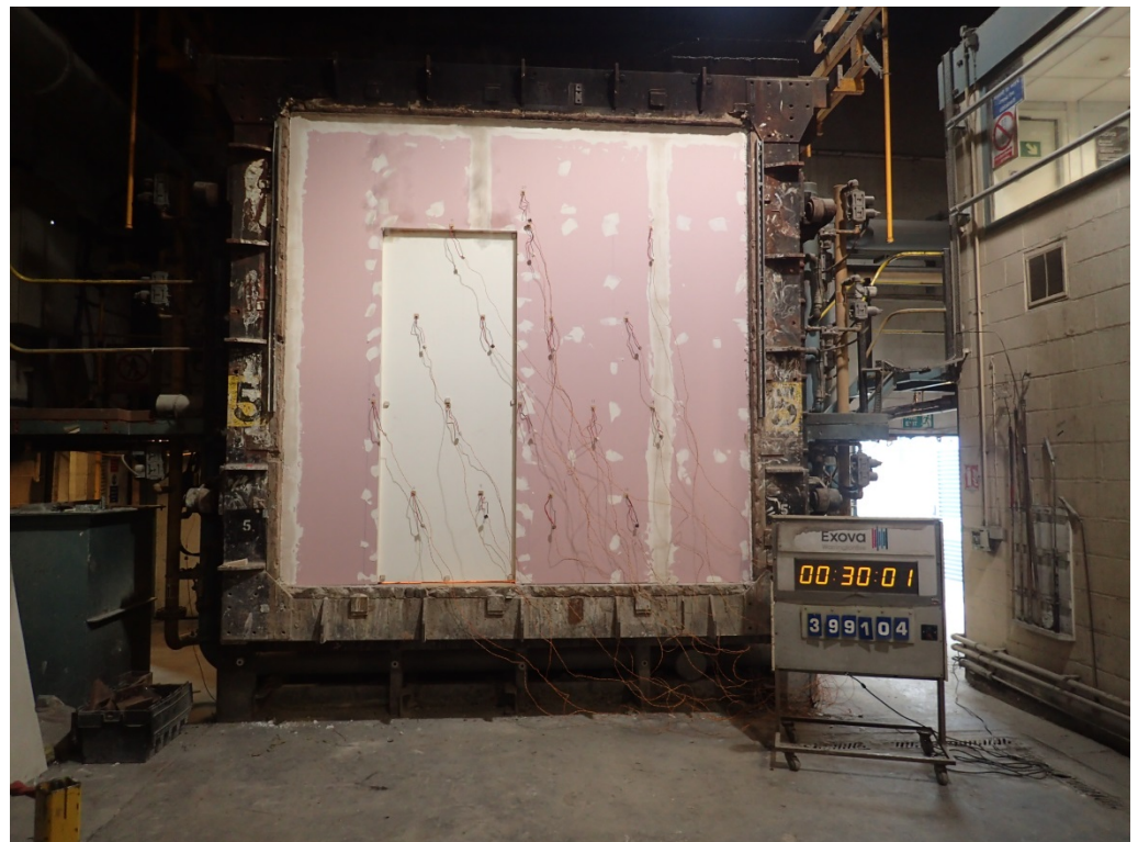
The unexposed face of the test construction after a test duration of 30 minutes
