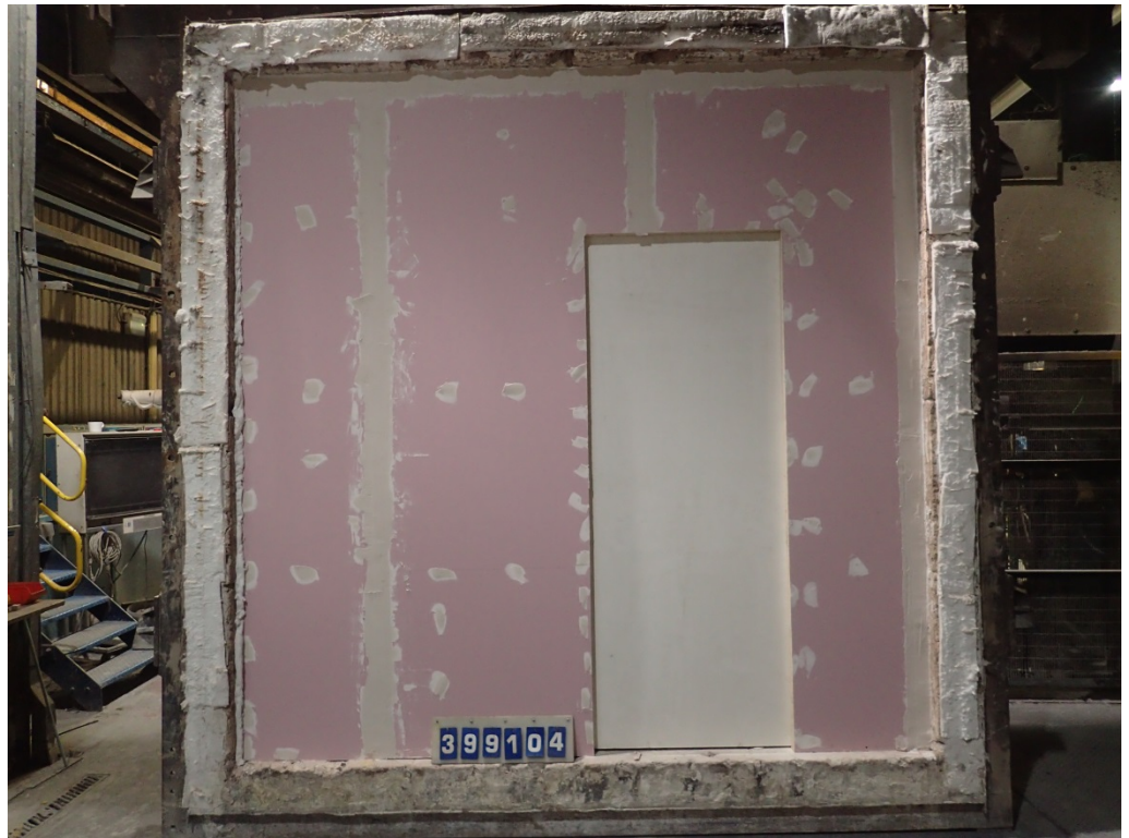
The exposed face of the test construction prior to testing
