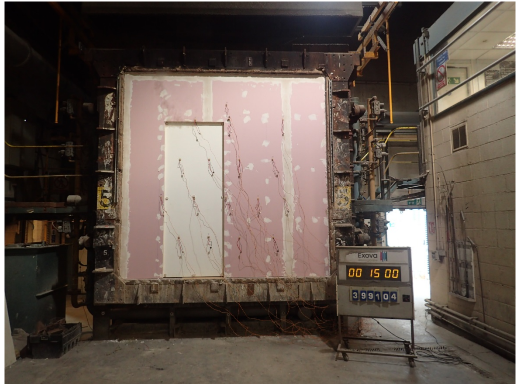
The unexposed face of the test construction after a test duration of 15 minutes
